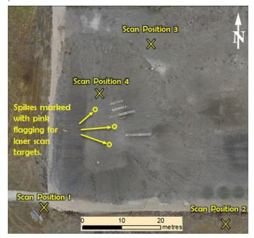
**Figure 3** TLS scan positions and spikes used for the registration
