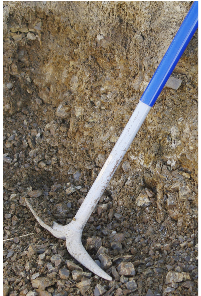
Figure 7 Odonah Member of the Pierre Shale Formation: A hard olive-grey siliceous shale with mean relative density (specific gravity) of 1.8 Photography: R.A. McGinn
